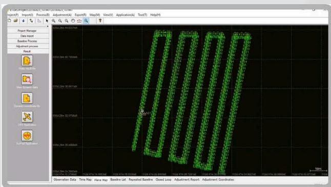
Geosolution features a dedicated UAV module for a quick and easy workflow in computing GNSS data from UAV-survey missions. The powerful UAV module allows trajectories to be processed quickly, and visualisation of the collected and post-processed data on a single interface.
