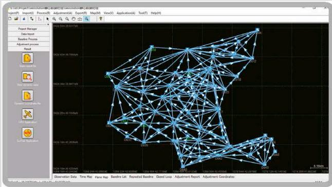
Geosolution's proprietary algorithm can process baseline vectors and adjust any 2D/3D static network quickly and accurately. No matter if it is a network with a single loop path or a complex network with interconnected paths, Geosolution can fit all the observed data simultaneously and provide the best solution.
